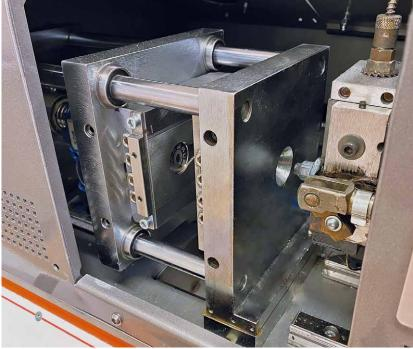
INJECTION MOULDING line is designed to test colours, polymers, and additives. It can also be used to prepare specimens for analytical purposes with low waste and energy consumption.
