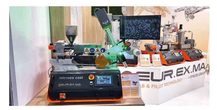
CAST FILM lines are designed for the quality control of polymers, compounds, masterbatches, and recycled materials. The film samples can be used for mechanical properties testing, visual control of defects, processability of polymers and color matching.
