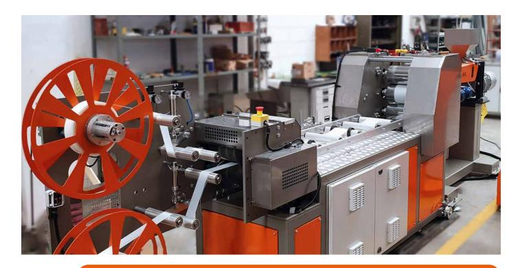
FOIL/SHEET lines are designed for the quality control of compounds and recycled materials. The samples can be used for mechanical properties testing, visual control of defects, processability of polymers, colour formulas and thermoforming.
