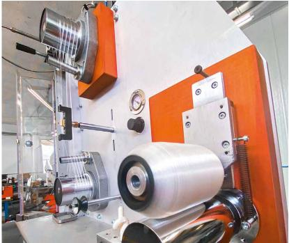
MELT SPINNING line is designed for the creation of continuous filament and Full-Drawn Yarn samples used to test several kinds of polymers.
