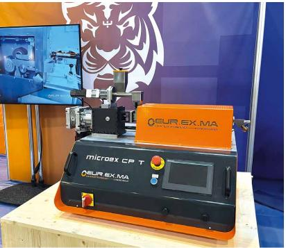
COMPOUND lines are designed to test different formulations of compounds or small batches of additives and colour masterbatches with low cost and waste.
